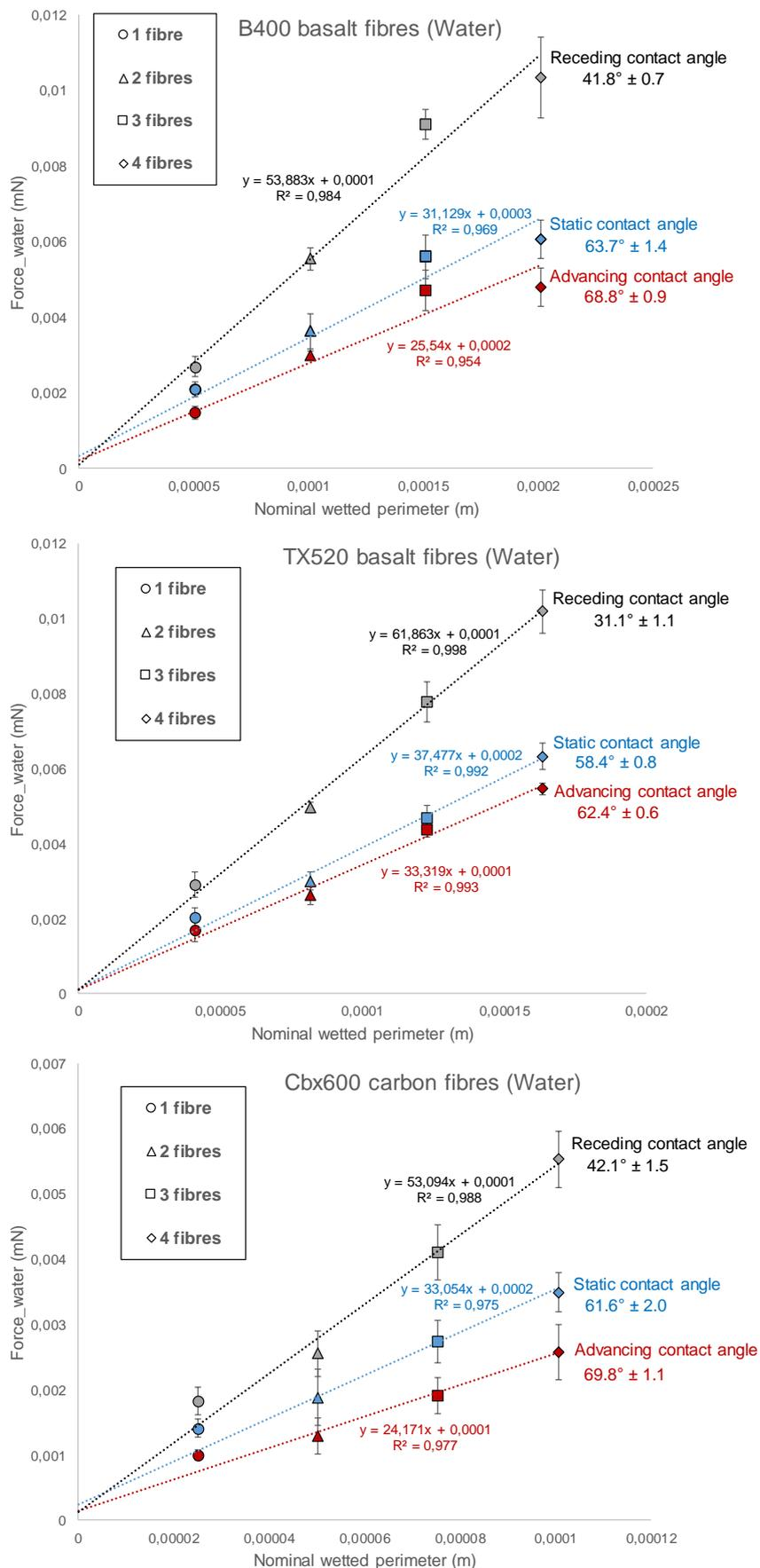
**Figure 5.** Measurements of contact angles in water for B400 basalt fibres, TX520 basalt fibres and Cbx600 carbon fibres
