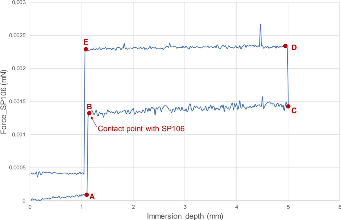
**Figure 3.** Example of a complete cycle for one B400 basalt fibre in SP106 resin with the K100SF tensiometer.
