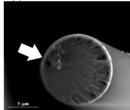
(c) Heat treated at 600°C for 35 min
