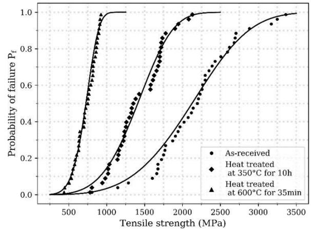
**Figure 3.** Weibull distribution of basalt fibers – before and after desizing. For each condition, the experimental data are represented by markers and the two-parameter Weibull distribution by a continuous line.
