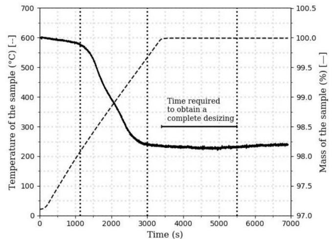
**Figure 1.** Mass variation of basalt fibers measured by TGA. The as-received fibers were heated at a rate of 10°C.min<sup>-1</sup> up to 600°C and were maintained at this temperature for 1 h in air
