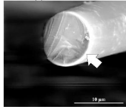
(b) Heat treated at 350°C for 10 h
