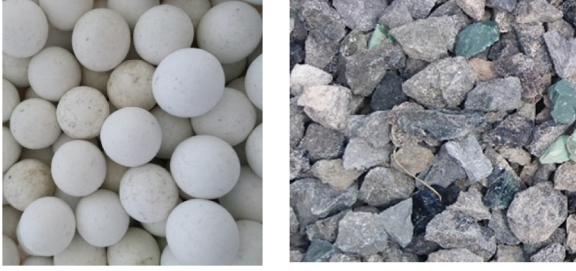
Regular 2cm spheres Alumina Irregular 2cm average rocks Cofalit®
