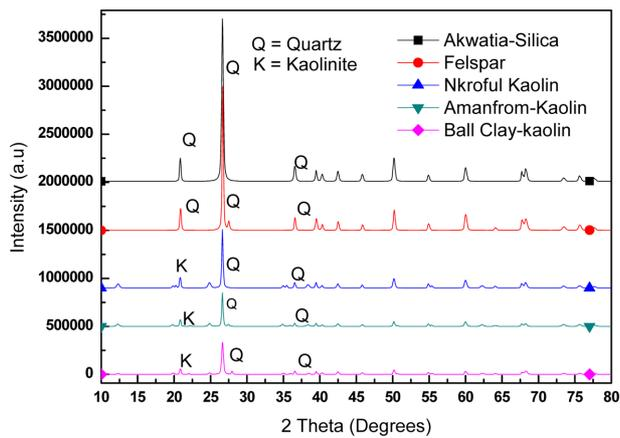
**Fig. 3.** X-ray diffraction patterns of the various samples.
