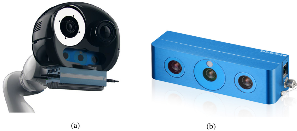
Fig. 1 (a) Robot-based inspection system with three cameras mounted on an end effector and (b) Ensenso N35 3-D sensor.
