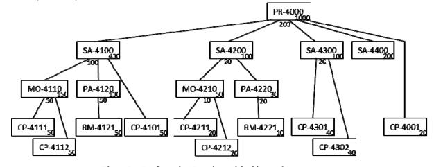
Figure 2 - Configuration Generic model with cost data
