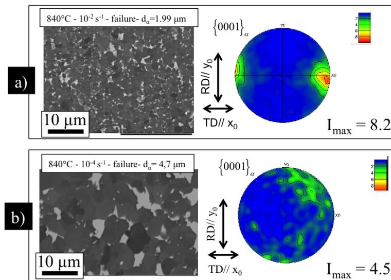
Figure 6: SEM-BSE images and  $\{0001\}_\alpha$  pole figures of the FG material after tensile tests at 840°C and for two different strain rates :
