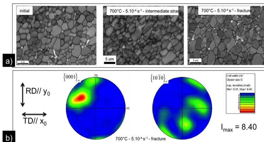
Figure 4: (a) band contrast images showing the microstructure of the FG material tested at 700°C with a strain rate of  $5.10^{-4} \text{ s}^{-1}$  and for various strain (from initial to the failure) (b) pole figures obtained for the FG material after tensile test (700°C /  $5.10^{-4} \text{ s}^{-1}$ )
