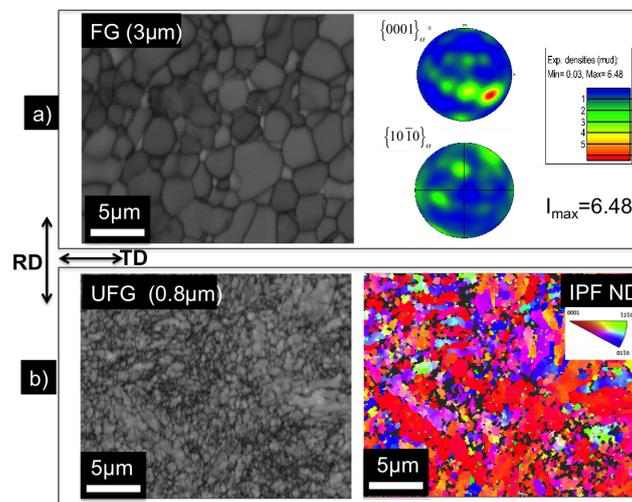
Figure 1: initial microstructure of (a) the fine grained (band contrast images and pole figures from EBSD data) and (b) the ultra-fine grained Ti6242 (band contrast images and IPF ND maps from EBSD data) (RD, TD and ND are respectively the Rolling, Transverse and Normal directions of the sheet)
