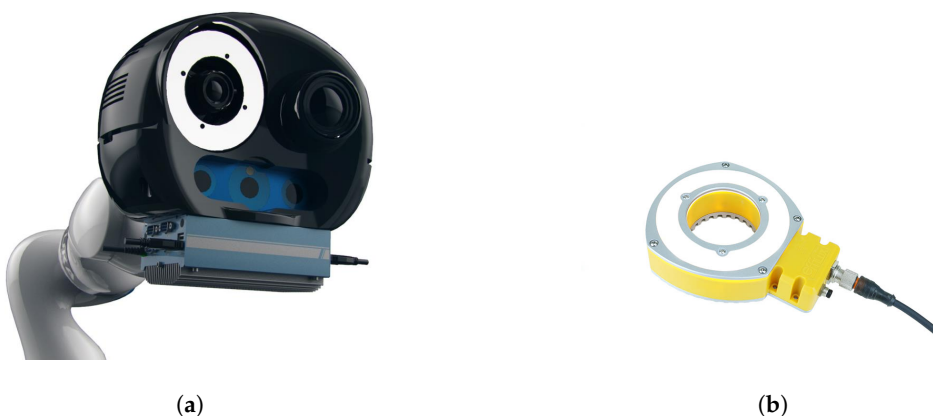
Figure 2. (a) Vision-based sensory system mounted on the robot; (b) additional lighting around the inspection camera.
