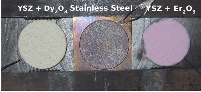
Fig. 12. Multi-material part: on the left is a sample of stainless steel substrate coated with a 200\mu\text{m} layer of zirconia powders mixed with dysprosium oxide ( \text{YSZ} + \text{Dy}_2\text{O}_3 ), in the middle is the stainless steel sample, and on the right is a sample of stainless steel substrate coated with a 200\mu\text{m} layer of zirconia powders mixed with the Erbium oxide ( \text{YSZ} + \text{Er}_2\text{O}_3 ).
