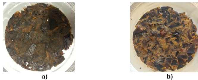
FIGURE 3. The pressed cake condition at a) 92 °C and b) 66 °C
