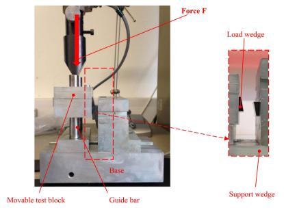
Figure 3. Shear device.
