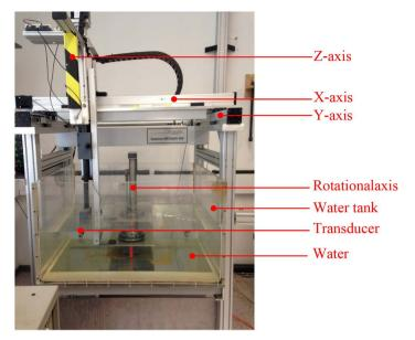
Figure 1. Ultrasonic device.
