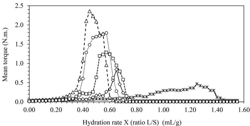
Fig. 3. Mean torque variation in mixer torque rheometer (MTR-Caleva<sup>®</sup>) during wet agglomeration of different flours. (—\*— Corn, —△— Amaranth, —□— Buckwheat, ...○... Quinoa).
