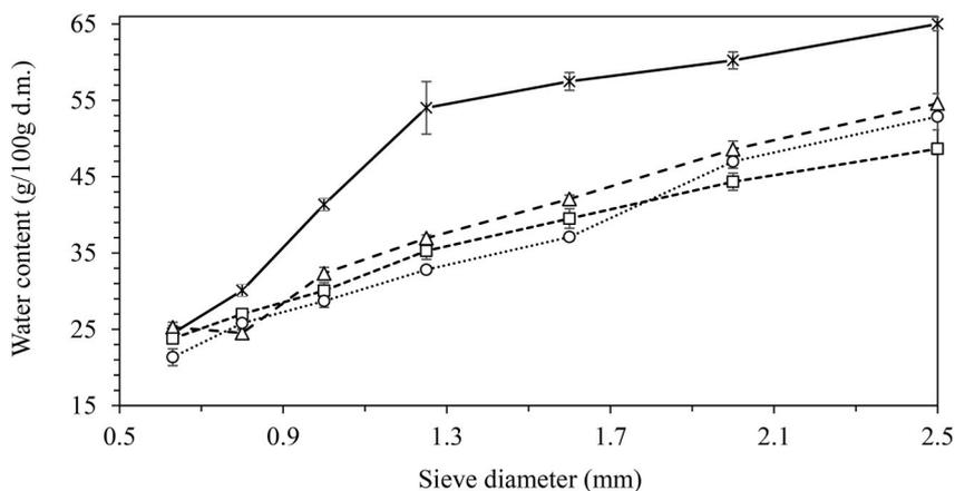
**Fig. 4.** Water content of the different diameters of wet agglomerates produced by the different flours on Mi-Pro<sup>®</sup> granulator. (—\*— Corn, —△— Amaranth, —□— Buckwheat, ...○... Quinoa).
