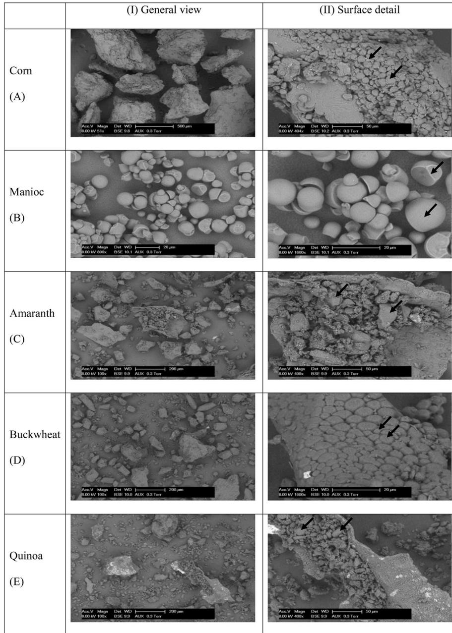
Fig. 2. Characterization of general view of particles (I) and their surface detail (II) by scanning electron microscopy for raw flours; (A) corn, (B) manioc, (C) amaranth, (D) buckwheat, and (E) quinoa. Starch grains are showed with arrows (→) in surface detail.
