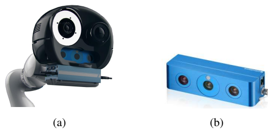
Figure 1: Acquisition system: (a) Robot with its vision-based sensory system, (b) Ensenso N35 3D scanner
