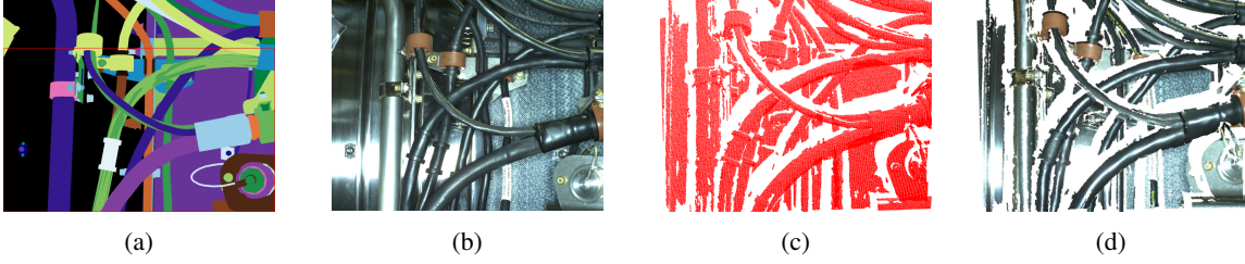
Figure 3: Example of our dataset. (a) CAD model, (b) 2D image, (c) 3D point cloud and (d) 3D point cloud with texture
