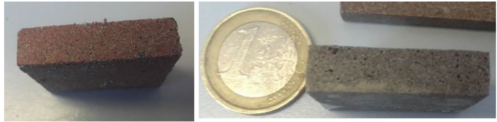
Fig. 5 Sintered plates samples (40 and 20% wt clay on the left and right respectively) fired at 1125 °C. The closed porosity of the 1125-20 sample is obvious
