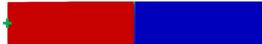
Figure 2: Initial state of the cylindrical squeeze-flow model, with the position of the pressure results shown Figure 3 indicated by a cross.
