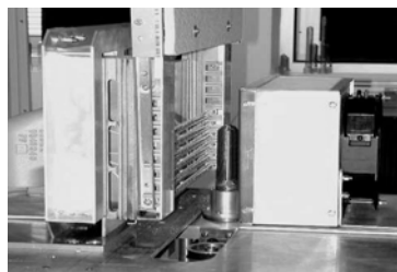
Figure 2 : Experimental setup, the infrared oven
