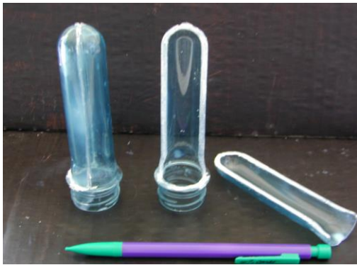
Fig. 9 Preform longitudinally cutted
