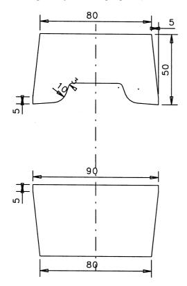
Fig. 6. Geometry of the tools (dimensions: mm).
