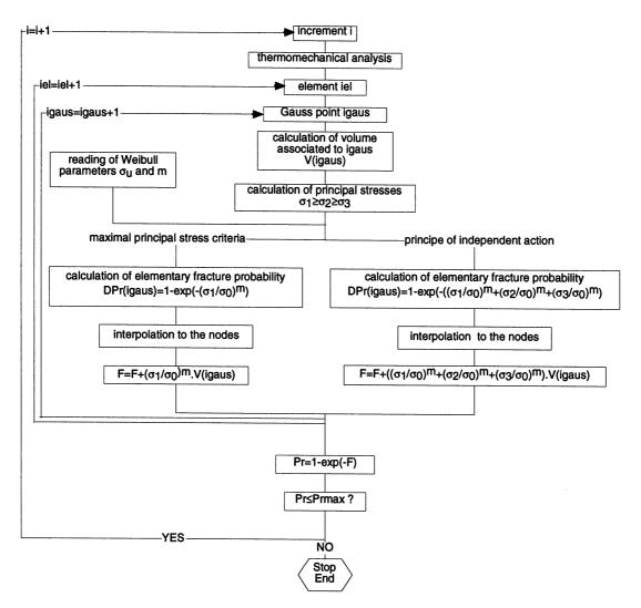
Fig. 1. Computational elements of the failure-prediction routine.
