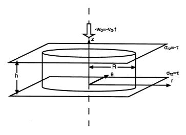
Fig. 2. A cylindrical workpiece pressed between two planes with uniform friction.
