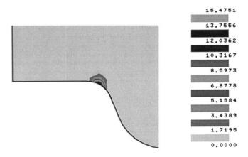
Fig. 9. Local risk of rupture (%) of the upper tool around the engraving fillet radius.
