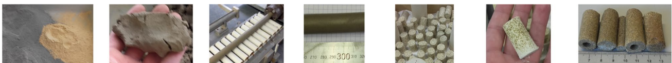
Fig. 1 Stages of the production process. From left to right: dry powders before mixing, paste formation, extrusion, extruded green body, fired batch and individual piece, fired cylinders prepared for analysis
