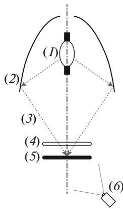
**Fig. 1.** Experimental apparatus schematics [6]. (1) 4 kW xenon arc lamp, (2) elliptical mirror, (3) a ray, (4) removable quartz window, (5) screen, (6) camera.
