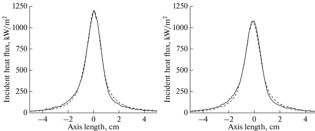
**Fig. 3.** Heat flux distributions at the focal spot without additional window (on the left) and with additional window (on the right). Continuous line: along  $x$  axis, dashed line: along  $y$  axis.
