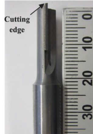
Fig. 2. PCD tool used with two straight flutes.
