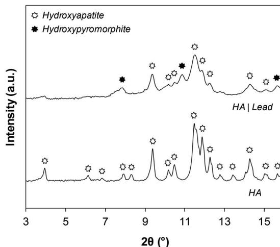
**Fig. 9.** Stacked plot of the X-ray diffraction patterns of the hydroxyapatite and the hydroxyapatite after the removal of lead (HA | lead) obtained using a silver radiation source.
