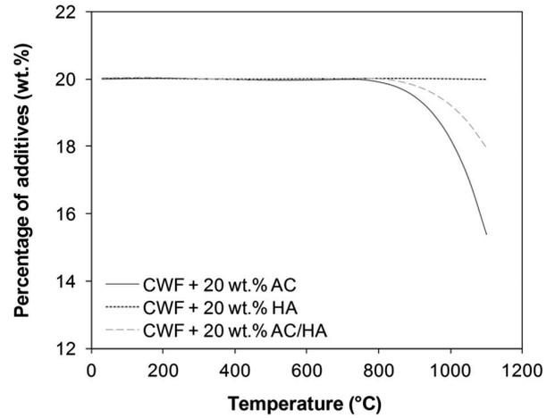
Fig. 2. Dependence of the percentage of additives on the firing temperature of the ceramic water filter (CWF) with 20 wt.% addition of AC, HA, or AC/HA. Data were obtained using TGA analysis.
