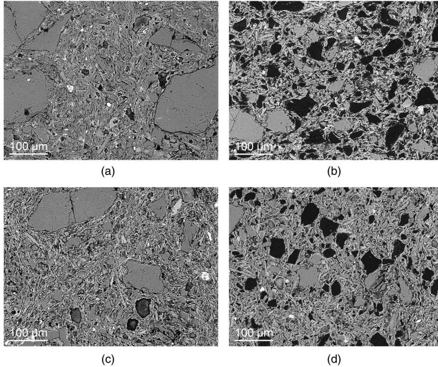
**Fig. 3.** SEM micrographs of (a) CWF without additives; (b) CWF with 20 wt.% addition of activated carbon; (c) hydroxyapatite; and (d) activated carbon and hydroxyapatite after firing of the ceramic water filters at 950°C in an air atmosphere.
