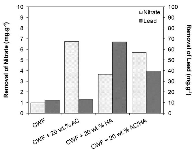
**Fig. 7.** Efficiency of the CWF without additives and the CWF with 20 wt.% addition of AC, HA, or AC/HA in the removal of nitrate and lead. Data were obtained using ion chromatography (IC) and inductively coupled plasma mass spectrometry (ICP-MS).
