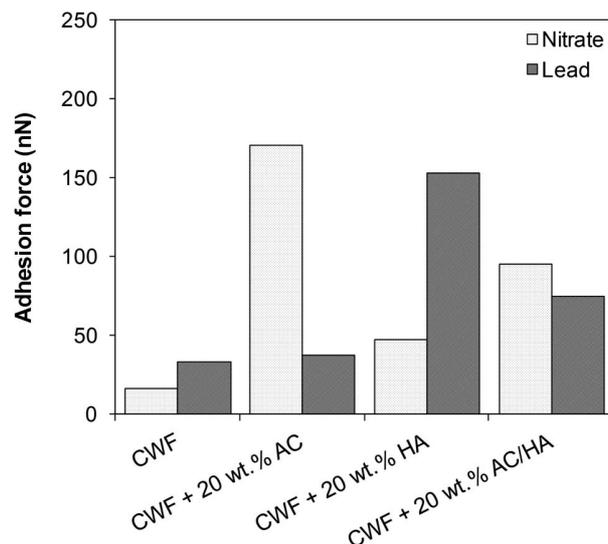
**Fig. 6.** Adhesion forces between the contaminants (nitrate and lead) and the CWF without additives and the CWF with 20 wt.% addition of AC, HA, or AC/HA. Data were obtained using atomic force microscopy (AFM).
