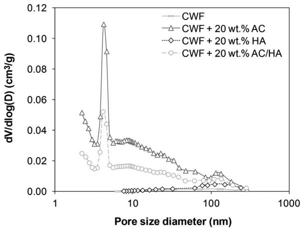
**Fig. 4.** Pore-size distribution of CWF without additives and CWF with 20 wt.% addition of AC, HA, or AC/HA after firing of the ceramic water filters at 950°C in an air atmosphere. Data were obtained using nitrogen adsorption analysis and the BJH method.
