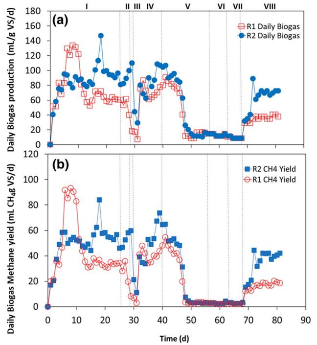
Fig. 2 Dynamic changes of **a** daily biogas production (mL g<sup>-1</sup> VS day<sup>-1</sup>), and **b** daily methane yield (mL CH<sub>4</sub> g VS day<sup>-1</sup>) in the process of FW AD under mesophilic condition
