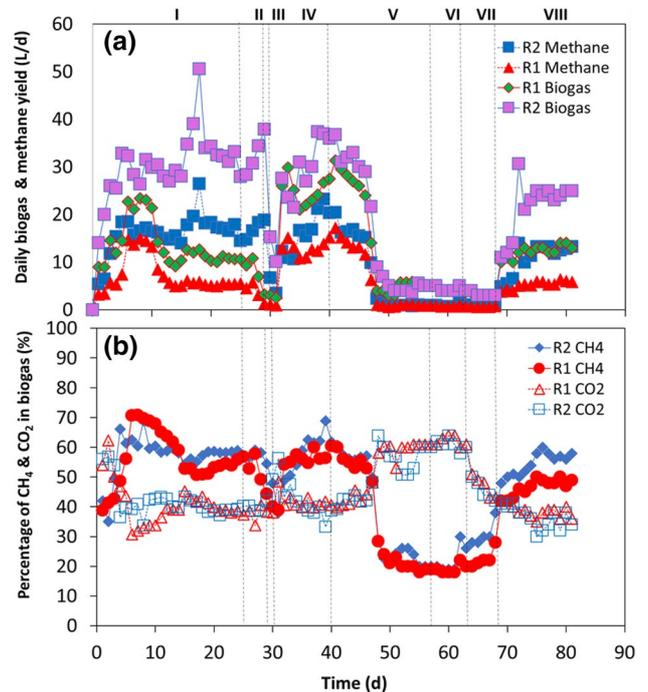
Fig. 3 Dynamic changes of **a** daily biogas production and methane yield (L day<sup>-1</sup>) of the two-reactor's combined, and **b** daily CH<sub>4</sub> and CO<sub>2</sub> composition (%), in the process of FW AD under mesophilic condition
