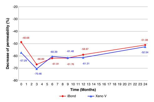
Fig. 2. A representative curve of the permeability for 2 years after application of the adhesive systems.
