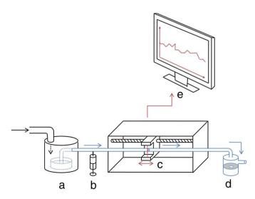
**Fig. 1.** Hydraulic conductance experimental set-up. The components are a) the pressurized reactor to reach 0.2 bars on a physiological solution pouch; b) a syringe for insertion of an air bubble; c) the Flodec bubble motion analyzer; d) the sample holder where the liquid phase penetrates the dentin slab to be tested; and e) the data recovery and analysis system.
