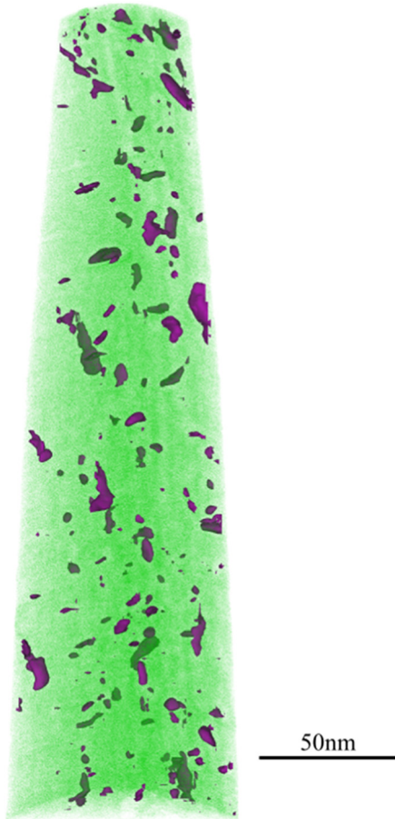
Fig. 12. Three-dimensional APT reconstruction of Ni atoms (green) of a sample tempered at 516 °C for 10 h. Carbides are represented as violet isoconcentration surfaces (total concentration of Mo and C is 36 at. pct). (For interpretation of the references to color in this figure legend, the reader is referred to the web version of this article.)
