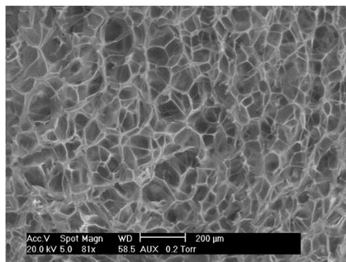
Figure 3: SEM images of samples at T<sub>5</sub>=135 °C, T<sub>6</sub>=115 °C, CO<sub>2</sub>=7.3 %, N=20 rpm.
