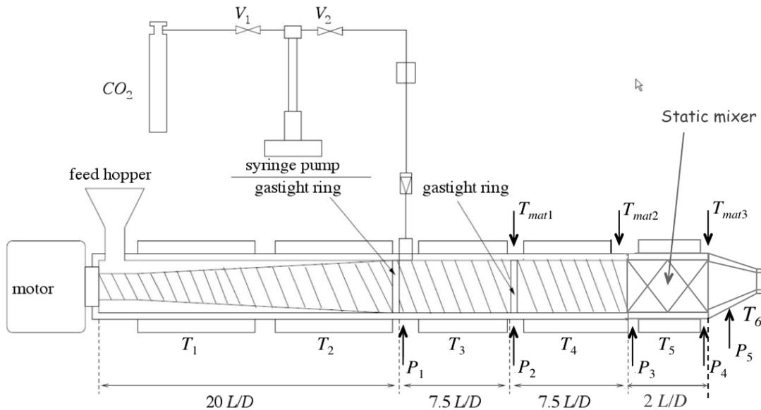
**Figure 1: experimental device.**
