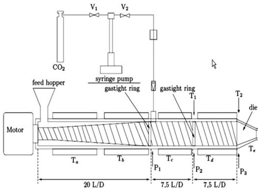
ScCO<sub>2</sub>-assisted extrusion of a mixture of active molecule and Eudragit E was performed on a single-screw extruder (SCAMEX, Crosne, France), with a large L/D ratio of 35.
