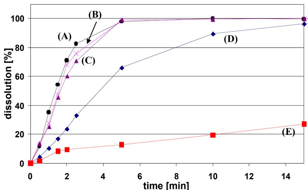
**Figure 5. Dissolution of Carvedilol from HME formulations (A, B, C, D) in comparison to unprocessed crystalline Carvedilol (E). (A) CO<sub>2</sub>-foamed-extruded and ground, (B) extruded and ground, (C) extruded, (D) CO<sub>2</sub>-foamed sample.**
