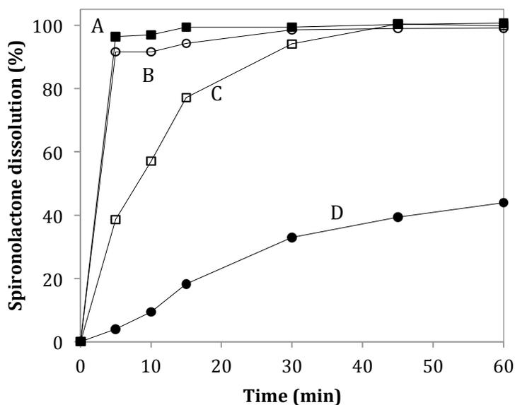
**Figure 6. Dissolution of Spironolactone from HME formulations (A, B, C) in comparison with unprocessed microcrystalline Spironolactone (D). (A, B) CO<sub>2</sub>-foamed-extruded and ground, (C) CO<sub>2</sub>-foamed sample.**
