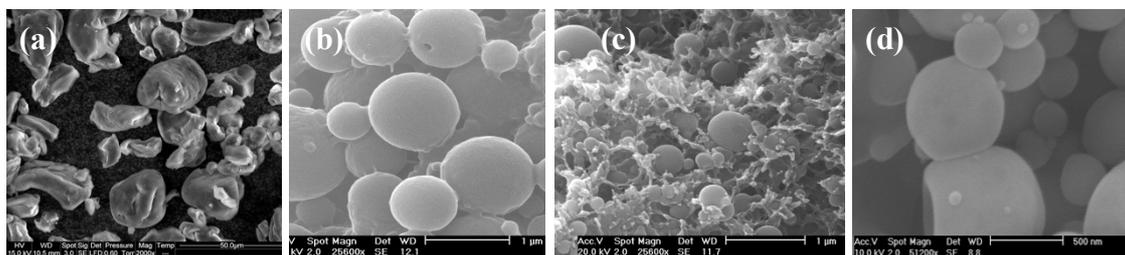
**Figure 1:** SEM photographs of commercial chitosan (a) and chitosan particles generated by SAS process for two potassium hydroxide concentrations (1% (b) and 2% (c)) and by SCASA process (d)
