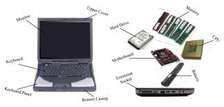
Figure 4. Predefined components of a laptop computer
