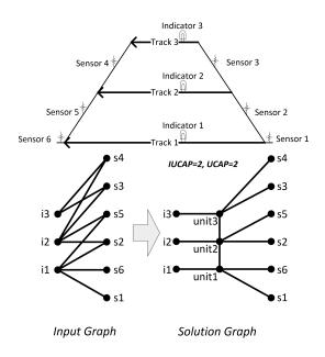
Figure 1. Railway track layout, PUP input and solution
