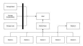
Figure 4. Graphical representation of how modules are dependent on each other. One and only one storage module can be selected at a time to avoid conflicts. Therefore the main module is dependent only one of the set of storage modules. However, for the market modules, one or all modules can be selected.
