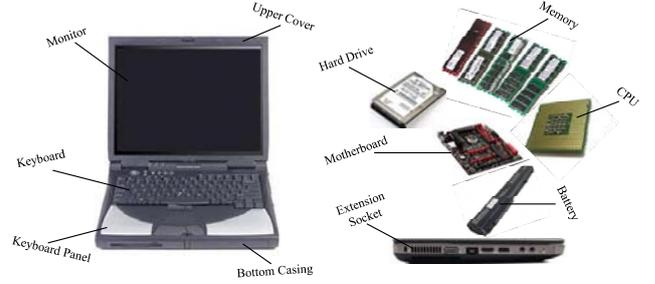
Figure 4. Predefined components of a laptop computer
