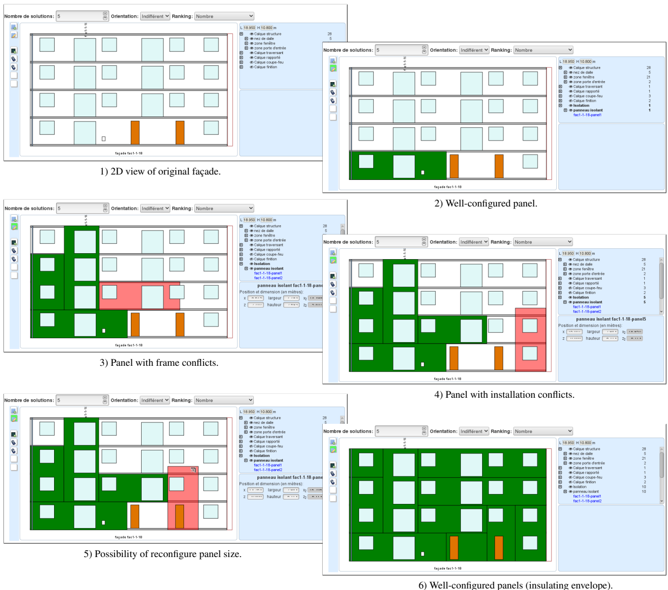
Figure 2. Demonstration: System actions through normal execution.
