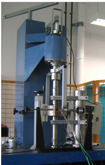
Fig. 1: Photo of the high load tribometer (equipped with a three-zone resistive furnace)
