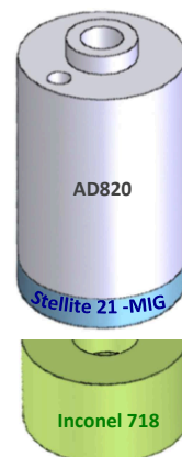
Fig. 2: Scheme of the tribological tests samples
