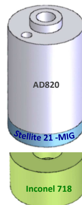
Fig. 2: Scheme of the tribological tests samples
