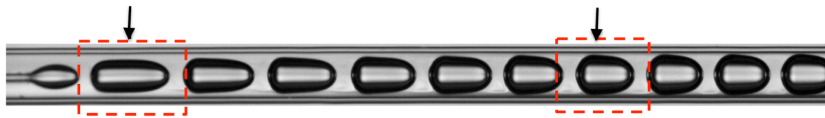
Figure 4: Decrease of the film thickness: in less than 2 cm it decreases from 23 to 1% of the inner diameter.
