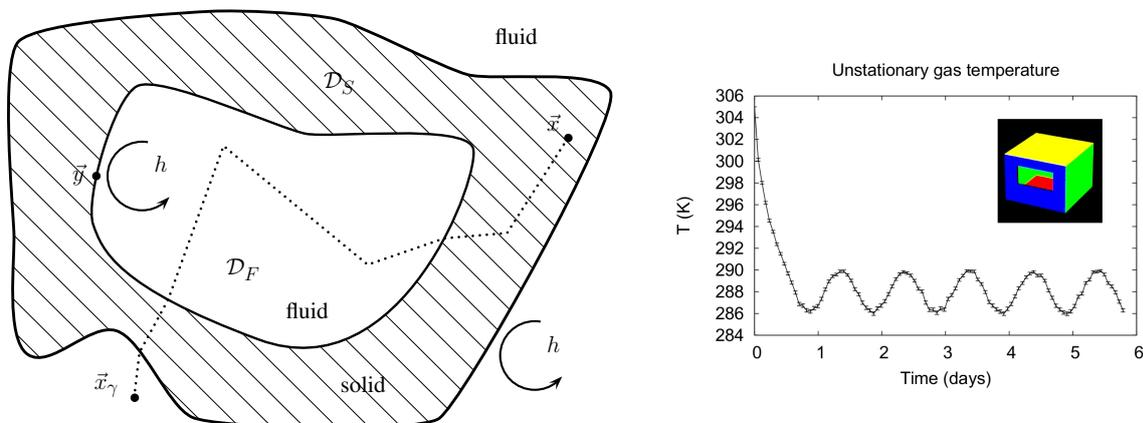
**Figure 1.** Fluid and solid domains (left). Academic example of a Monte Carlo simulation dealing with radiative, conductive and convective heat-transfers, for opaque solids and transparent fluids (internal air-temperature for a sinusoidal external forcing, right).
