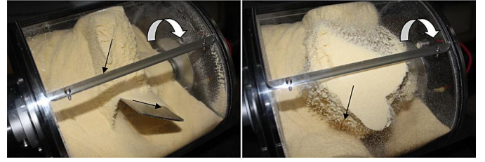
Figure 7. Rolling flow regime (left) and cataracting flow regime (right) for semolina inside the convective blender equipped with reclined blades.
