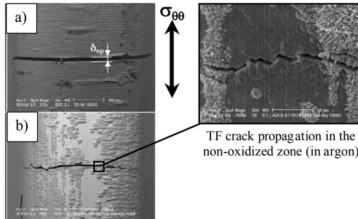
Fig. 8. Typical Uni-axial TF crack propagation ( $T_{\max} = 650^{\circ}\text{C}$ ):
