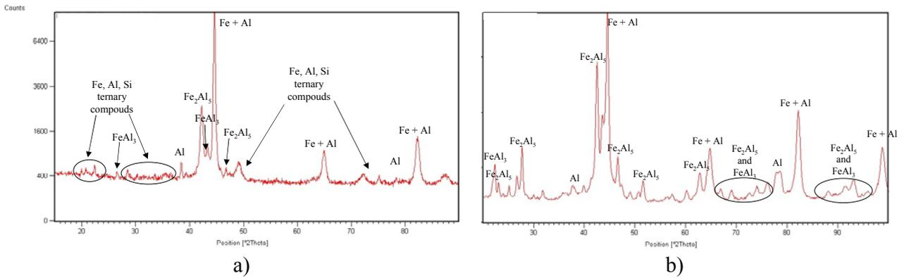
Fig. 5. X-ray diffraction pattern on X38CrMoV5 coupons :
