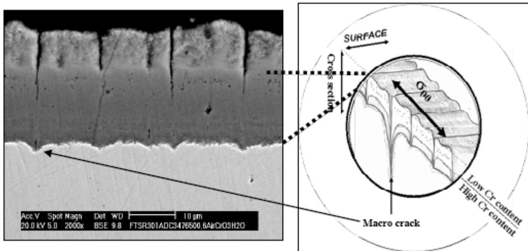
Fig. 9. Cross section of the edge tip of TF specimen tested at 650°C under air.
