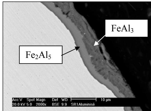
Fig. 6. Cross section of X38CrMoV5 steel aluminized at 550°C for 8h.
