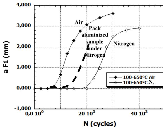
Fig. 10. Variation of cracks depth vs. number of thermal cycles under air and inert atmosphere for X38CrMoV5 with and without a pre-aluminized layer.
