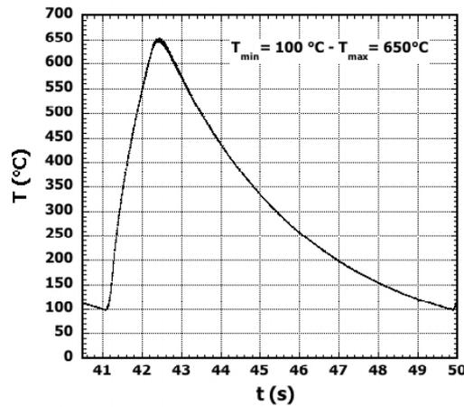
Fig. 3. Typical TF cycle at edge tip of specimens. Heating and cooling period are about 1s and 7s respectively
