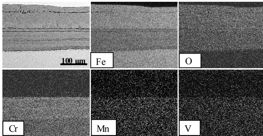
Fig. 1. X-ray maps of the cross section of an oxide scale grown during exposure at 700°C for 90 hours in wet air (pH<sub>2</sub>O = 198mbars)
