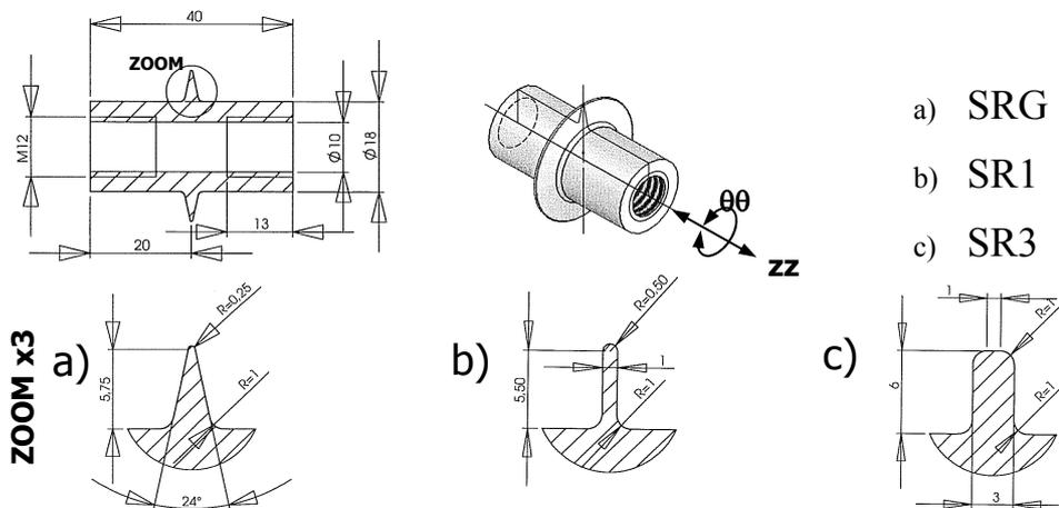
Fig. 2. Typical thermal fatigue specimens (dimensions: mm)
