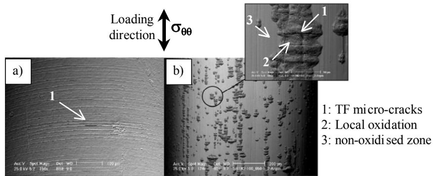
Fig. 7. Thermal fatigue oxidation mechanisms ( $T_{\max} = 650^{\circ}\text{C}$ ):
