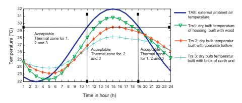
Fig. 5. Comparison of resultant dry bulb temperature of different housings.
