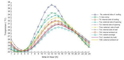
Fig. 2. Temperature profile with wood plank.
