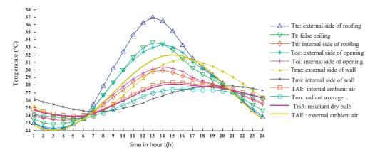
Fig. 4. Temperature profile with brick of earth and cement mortar.
