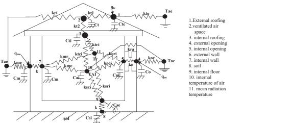
Fig. 1. Thermal node model of house and its electrical analogy.
