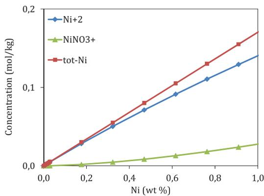
Fig. 3 Speciation of Ni using LLNL model
