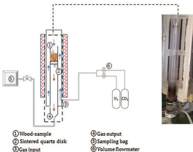
Fig. 1 Fixed bed Reactor
