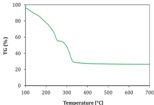
Fig. 7 Nickel nitrate degradation at 5 °C/min
