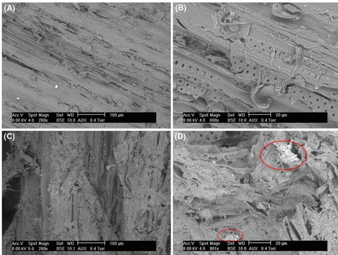
**Fig. 5** SEM images of raw wood (A, B) and the wood-5-Ni sample (C, D)
