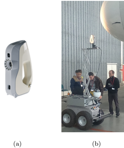
Fig. 5 (a) Artec Eva 3D scanner; (b) Air-Cobot with the scanner mounted on a pantograph
