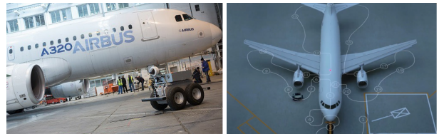
Fig. 2 (a) Air-Cobot and Airbus A320 airplane; (b) Illustration of moving map of Air-Cobot
