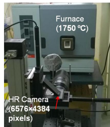
Fig. 8. High-temperature furnace with a high-resolution camera.
