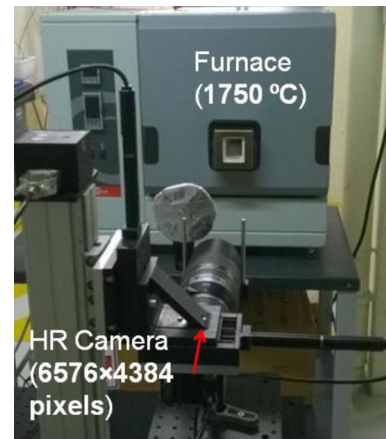
Fig. 8. High-temperature furnace with a high-resolution camera.
