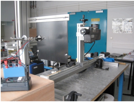
Figure 3 – Experimental set-up used for thermal conductivity measurement using IR camera
