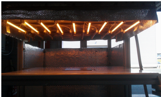
Figure 5 – Experimental IR heating oven and model schematisation
