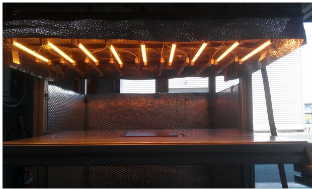
Figure 5 – Experimental IR heating oven and model schematisation
