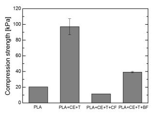
**Figure 7.** Compression strength of PLA foams.
