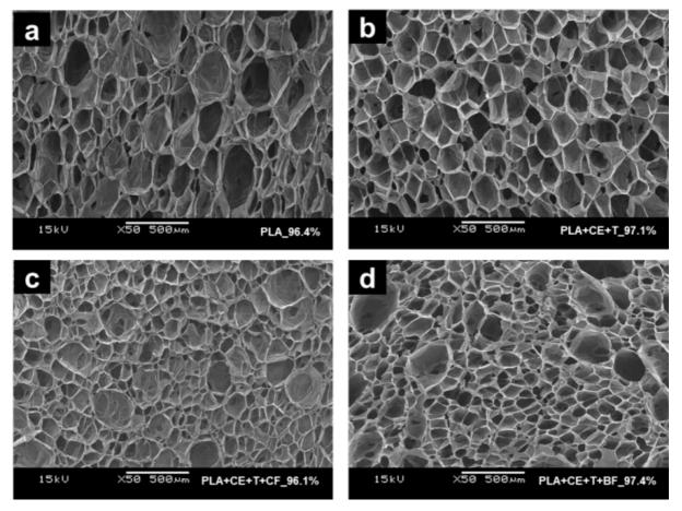
**Figure 4.** SEM micrographs of the cell morphologies obtained for highly expanded ( $\varepsilon$ >95%) PLA foams. The actual porosity values are represented after the abbreviation of the materials within every micrograph.
