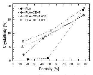
Figure 6. Foam crystallinity as a function of porosity
