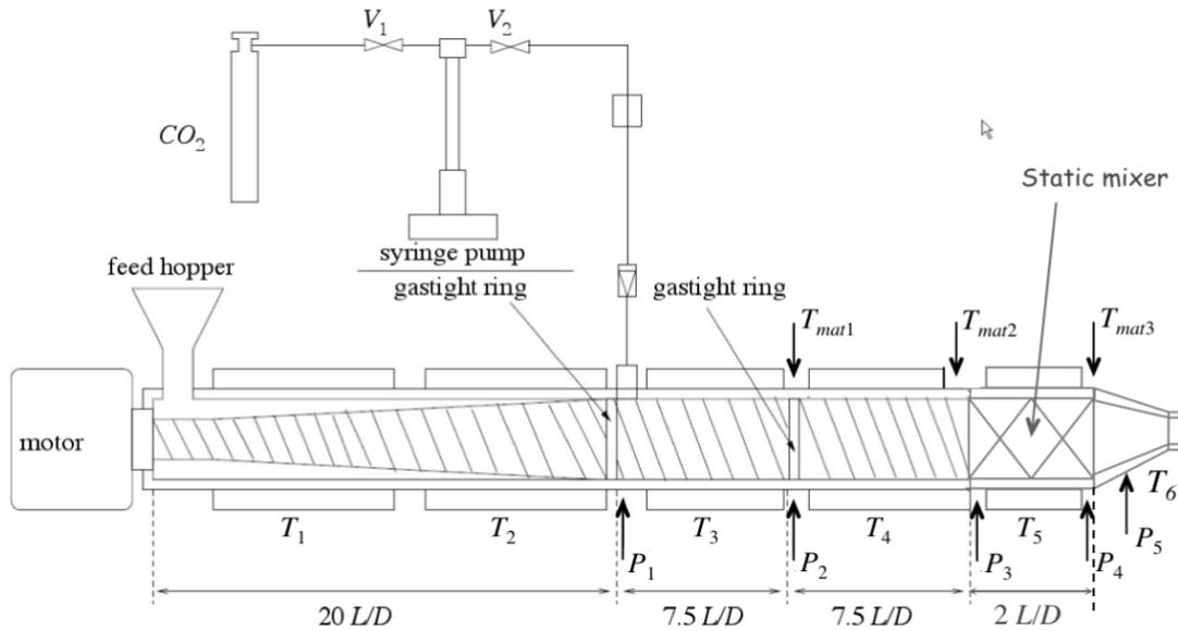
**Figure 1.** Schematic picture of the foaming system
