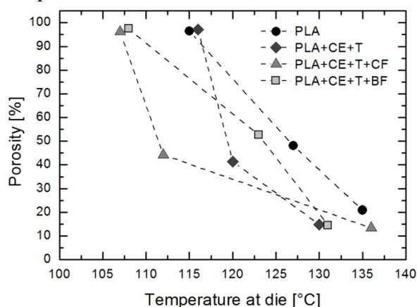
**Figure 3.** Effect of formulation and mixer and die temperatures on the porosity of PLA foams extruded at 8% of CO<sub>2</sub>
