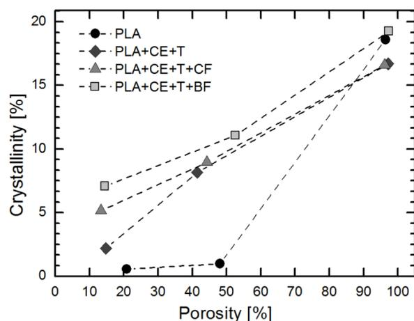
**Figure 6.** Foam crystallinity as a function of porosity
