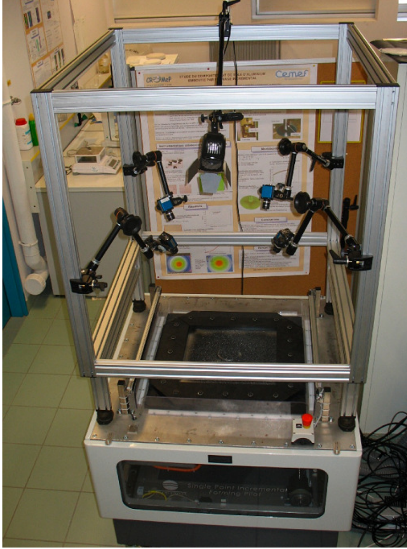
Fig. 3. The SPIF pilot instrumented with the 4-camera system.
