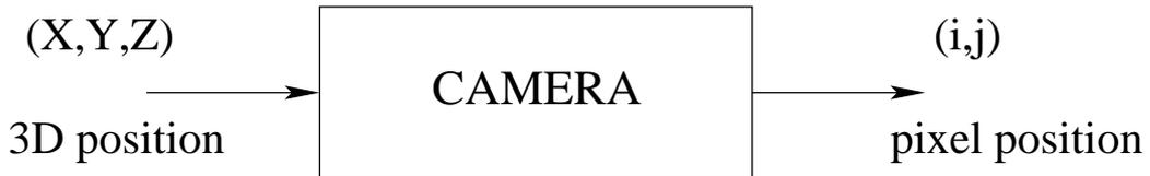
Fig. 5. From a geometric point of view, a camera converts a 3-D point  $(X, Y, Z)$  to a 2-D image point  $(i, j)$ .
