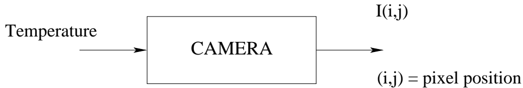
Fig. 1. From a radiometric point of view, a camera converts a temperature to a pixel gray level value I(i, j) .
