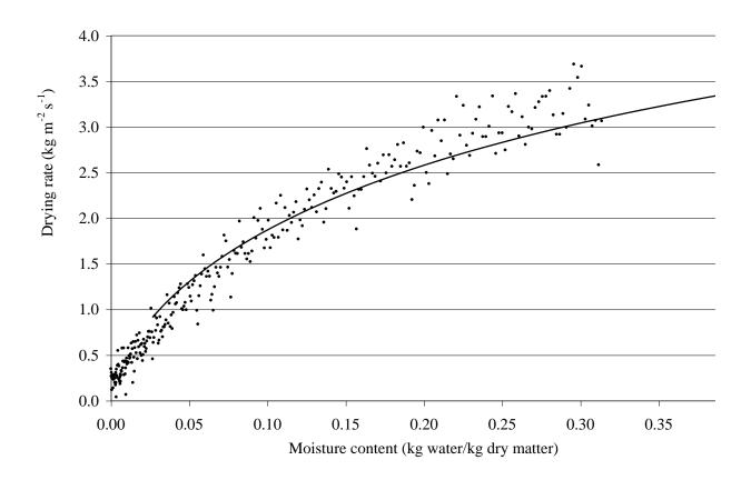
Figure 11 – Measured( — ) and adjusted ( — ) drying kinetics of the digested sewage sludge coming from Albi City ( $T_{wall}$  = 180°C,  $\omega$  = 40 rpm, d=1.15  $10^{-3}$ m).
