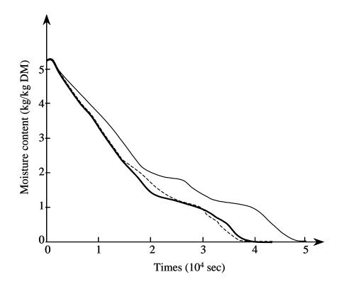
Figure 16 Measured (dot) and adjusted (line) drying kinetics of an anaerobically digested sludge ( (+), d=1.15  $10^{-3}$  m) and an extended aeration one (  $_{\bigcirc}$ ), d=0.9  $10^{-3}$  m) for  $T_{wall}$  = 160°C and  $\omega$  = 40 rpm.
